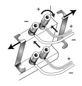
Figure 9. Loosen the terminals and remove the strapping bars that connect the two sets of terminals.
